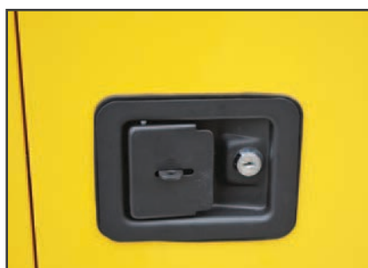
Recessed door handle with lock
