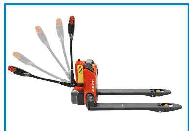
Handle is supported by an air spring so that the handle returns smoothly to the vertical position
