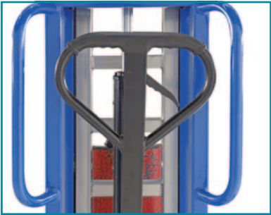
Handle lever to lower drum
